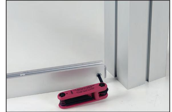
Detail A: Most horizontal extrusion connections have a patented expandable lock. This lock inserts into the groove of an opposing extrusion. Tightening the lock with the hex key tool expands the lock and creates a strong connection.
